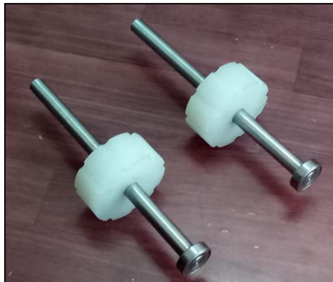
Fig: 5.7 Shaft with Sprocket and bearing mounted on it
