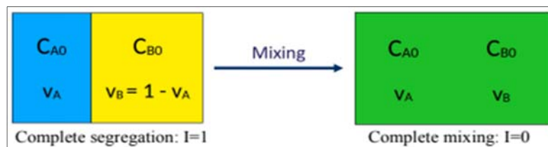
Figure 1.1 The concept of segregation [3]
